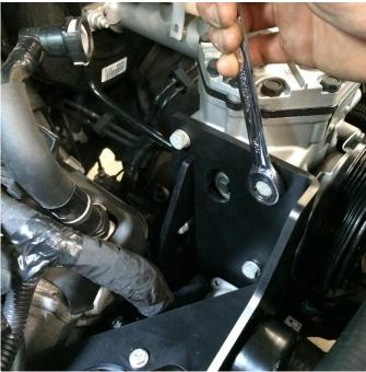
Four 3/8 bolts and lock washers are provided for mounting the compressor to the bracket. They should be tight but be careful not to strip the aluminum compressor body.
