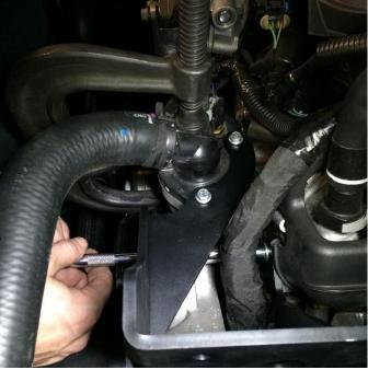
Loosely install the 2 supplied M6-1.0 x 35mm bolts through the bracket and into the thermostat housing. Then thread in the M8-1.25 x 25mm bolt through the bracket and into the head. These should be snug, but not tight.
