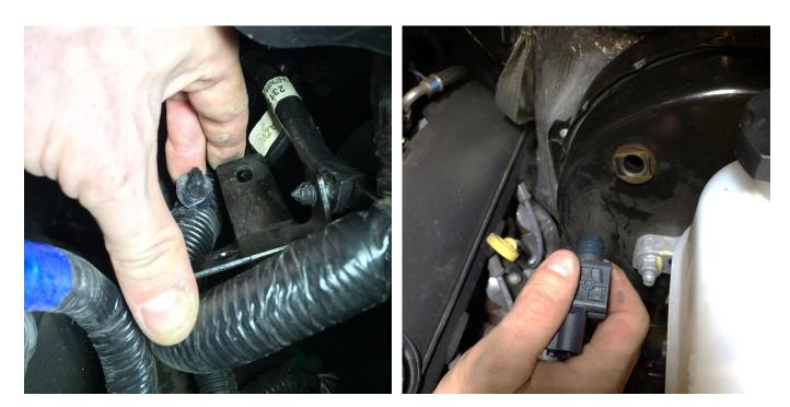
The bracket removed earlier can be disconnected from the wiring harness to allow the vacuum tube to be rerouted. The vacuum tube electrical plug can be disconnected, then it can be temporarily removed from the brake booster.
