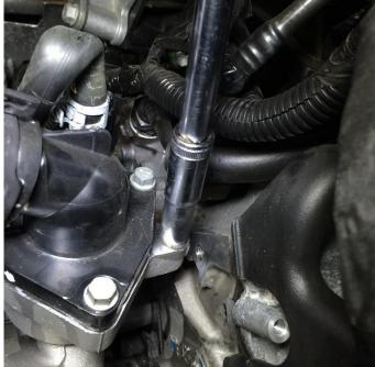
Remove the factory harness support as shown. Then remove the stud behind the thermostat housing.
