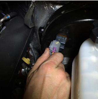
Reroute the vacuum tube so as to have more room from the exhaust manifold. Make sure that it does not rub any sharp corners of the bracket. Then plug it back into the booster and reinstall the electrical connector. Check to confirm the wires have room to the bracket and are not rubbing any sharp edges.
