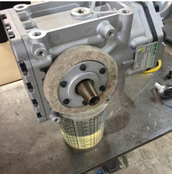
**Standard and SLM compressors:** Verify the new compressor has the half-moon shaped woodruff key installed in the crankshaft. **Standard Compressors only:** The compressors are shipped pre-filled with AC refrigerant oil, but it is recommended to run 12oz of SAE 30 non-detergent engine oil. Remove the screws from each side of the compressor fill ports and drain the oil.
