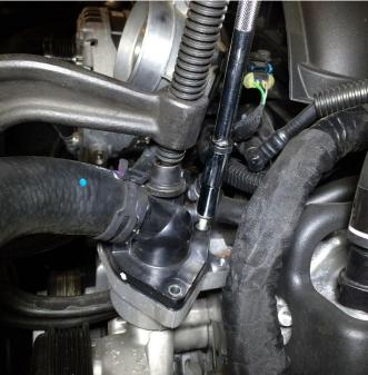
Place a C-clamp on the thermostat housing to prevent the loss of coolant while removing the 2 bolts shown. Loosen both bolts slightly and confirm the C-clamp is secure and that there are no leaks before completely removing the bolts.
