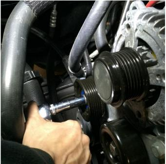
Insert the supplied M10-1.5 x 180mm bolt through the smooth idler pulley then through the 1.88" length stand-off and install where shown in **Image 18**. Insert the M10-1.5 x 50mm bolt through the grooved idler and the .30" length stand-off and install where shown in **Image 19**.
