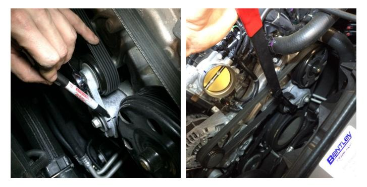
Start by making a witness mark across the tensioner pulley arm to indicate the factory belt tension. Then rotate the tensioner pulley to remove the belt.
