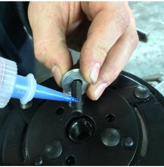
Install and tighten the 4 screws that attach the clutch. You can choose if you want the clutch wire oriented to the top or bottom. Install the 5/16 clutch retainer bolt and torque to **20-25ft lbs**. Never hammer the center bolt onto the snout. Let the screw pull it up until it seats.
